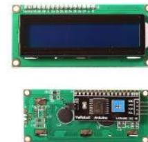
Gambar 2.4. Liquid Cristal Display (LCD) dan Inter Integrated Circuit (I<sup>2</sup>C)
