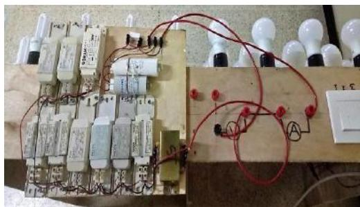
Gambar 10. Rangkaian filter pasif LC.
