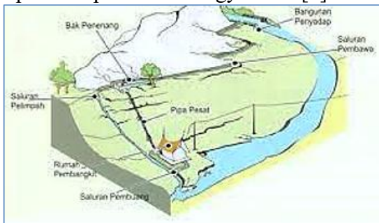
Gambar 2. 1 Skema PLTMH Sumber: https://bit.ly/3MgfnQW
