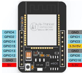
Gambar 3. Pin-out ESP32-CAM.
